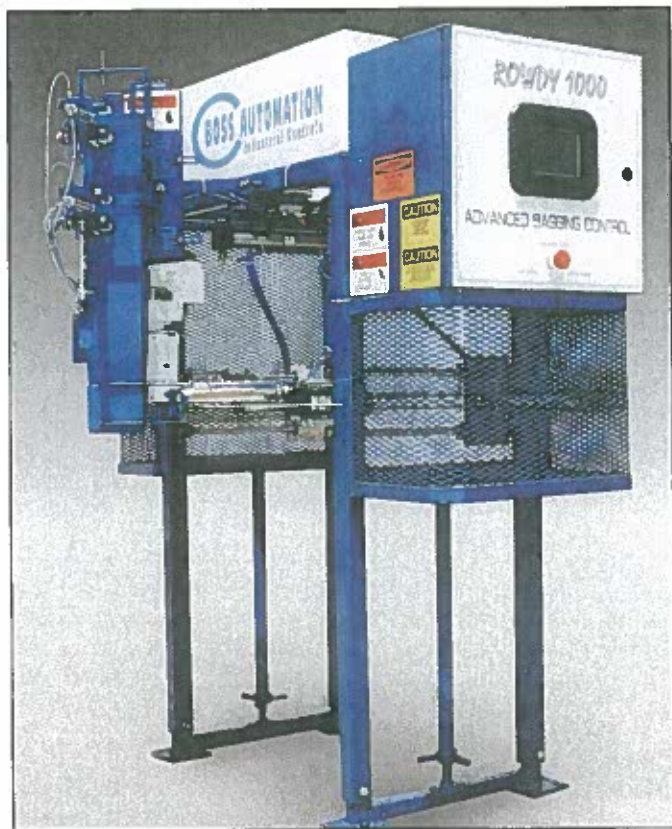
Boss Automation automated bag closer and tag placer to be installed at Richardson Seeds in Vega, TX.
